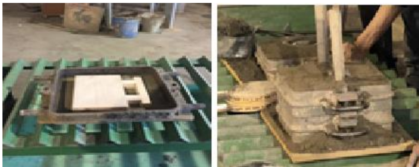
Figure 2. Drag and cope mold
